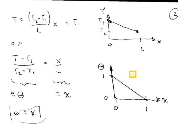
But recall  $g = -kA \frac{\partial T}{\partial n} = -kA \frac{\partial T}{\partial X}$   $= -kA \frac{(T_2 - T_1)}{L}$   $= \left(\frac{kA}{L}\right)(T_2 - T_1)$   $\delta T = gR_{therm}$   $g = \frac{(T_2 - T_1)}{R_{therm}}$   $So \left[R = \frac{1}{KA}\right] for well$  " How about 2 walls touching ...
